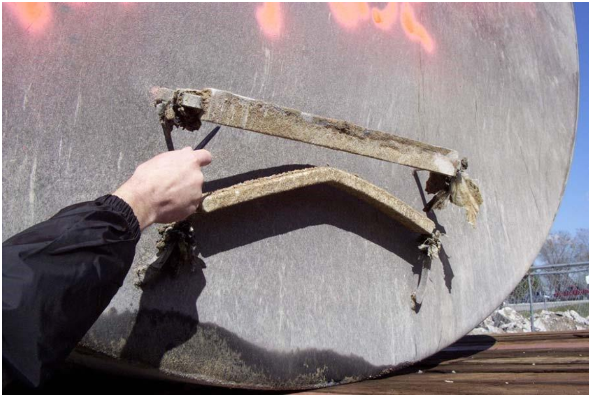
Used STIP-3 tank, showing the anodes.
