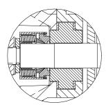
**SEAL DETAIL** Type 9, Mechanical, Self Lubricated. Carbon Rotating Face and Ceramic Stationary Face. PTFE Elastomers. Stainless Steel 316 Cage and Spring. Maximum Temperature of Liquid Pumped, 160°F (71°C).\*
