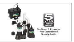
The side by side kit with primary and battery backup sump pump comes assembled complete with PVC pipe fittings and two check valves. The top outlet discharge is  $1 \frac{1}{2}$  PVC slip. Easily fits into standard sump basins with minimum diameter of 15".
