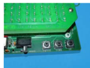
"Enter", "Up" and "Down" keys used to input data.
