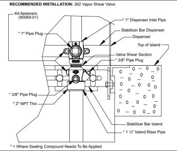
Figure 4: Shear Valve Installation
