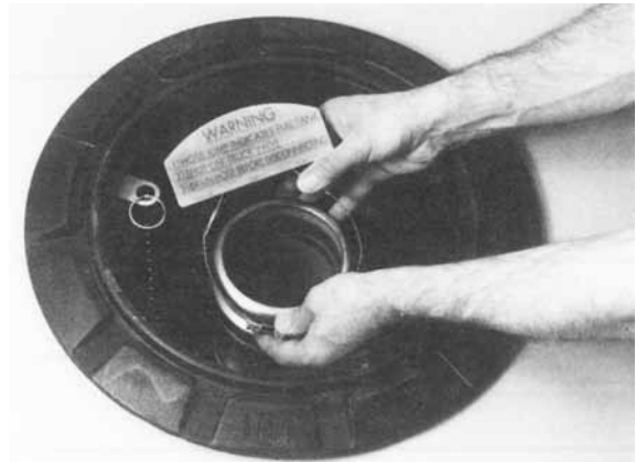
Figure 17: Install Warning Plate
