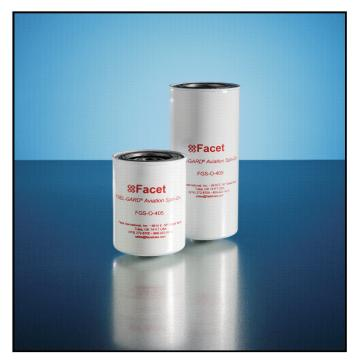
Facet's Fuel-Gard<sup>®</sup> Aviation Spin-On Filters perform three jobs to give you clean, dry fuel. They absorb free and emulsified water, remove ultra-fine solids even when surfactants and fuel additives are present, and shut down system flow when hit with a localized slug of water. The filters are designed to flow at a rate of 13 gpm (FGS-O-405) and 15 gpm (FGS-O-409).
