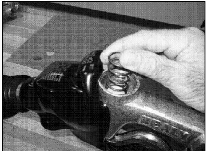
Figure 6: Installing New Spring
