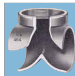
OPW-ES 464 Cast aluminum tee with female threads. Especially designed for handling jet fuel. Prevents high-velocity impingement on bottom of tank to reduce possibility of ignition of jet fuel. Available in 3" and 4".
