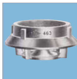
OPW-ES 463 Cast aluminum with female threads for 3" or 4" liquid loaders. Vertical wing ribs prevent drop tube from rising when filling. Accelerates discharge and prevents roiling of product when used on pressure discharge line.
