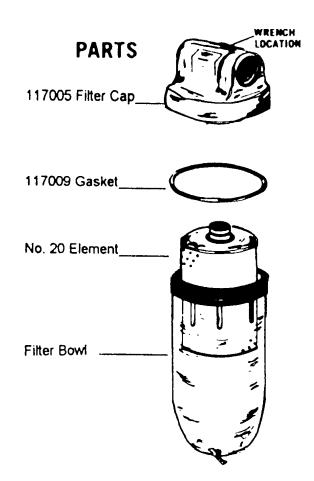
Visually check filter element for replacement. Change filter element when dirty or when flow is restricted. To replace filter element, unscrew filter bowl and unscrew filter element and replace. **Hand Tighten Only.**
