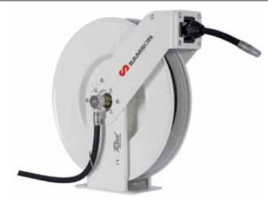
Heavy Duty reinforced double pedestal hose reel for air, low and high pressure water, medium pressure oil and high pressure grease. All metal construction, can handle up to 60' of 1/2" hose.
