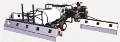
A hooded spray boom minimizes drift on windy days.
