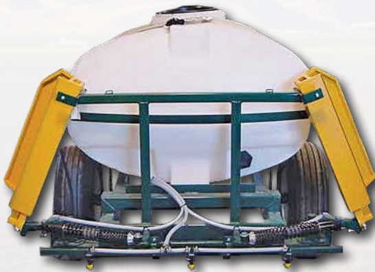
Boom shown in folded position.
