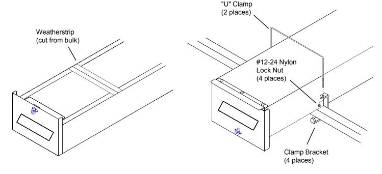
Figure 8. Assembly Weatherstripped for Crossmember
