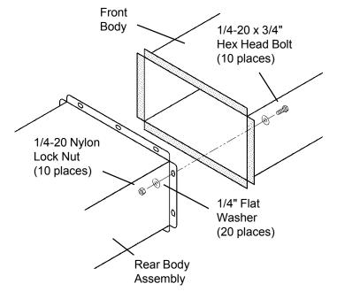
Figure 6. Rear Body Assembly to Front Body fastening
