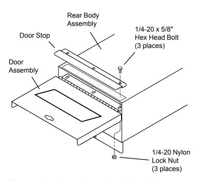
Figure 3. Door Stop and Door to Body Assembly
