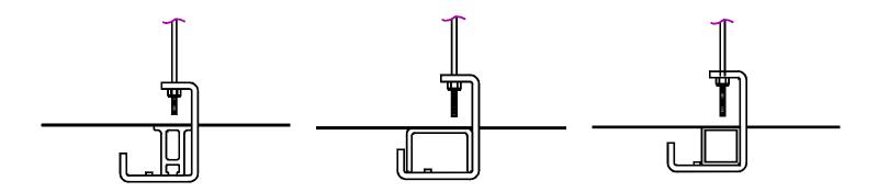
Figure 10a. Installation on a 211 aluminum crossmember
