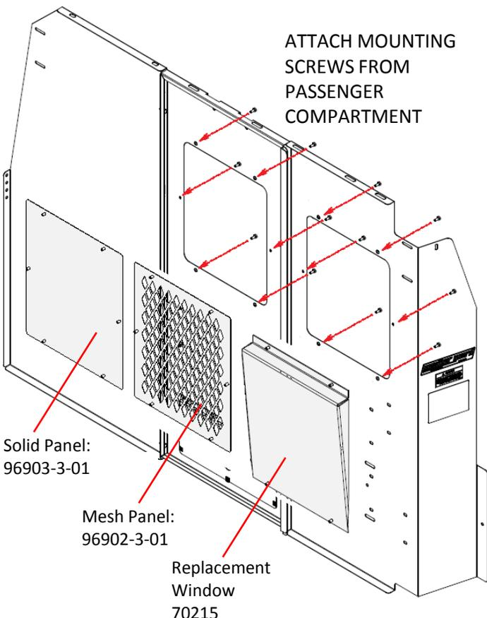
**STEP 1:** Remove existing windows from the bulkhead panels.
