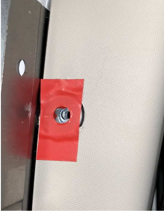
Step 8 Tape Spacers to B-Pillar Trim
