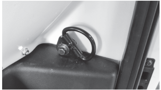
Passenger Side D-Ring (Cargo Side of Bulkhead)
