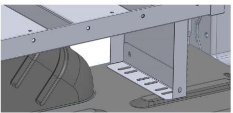
STEP 12. Slip the mounting foot from the other side of the end panel and install using 1/4-20 x 3/4" bolts, washers, and nylon lock nuts. Install to floor blind fasteners using 1/4-20 x 1-1/2" bolts. Repeat steps 11 and 12 until all mounting feet are installed. Note that you only need to use one mounting foot where the driver side shelves join.
