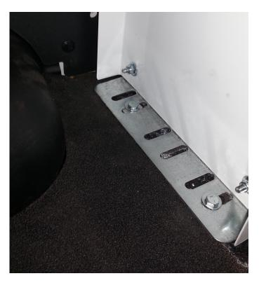
**STEP 13.** Torque down the 1/4-20 x 3/4" bolts, washers, and nylon lock nuts installed in **STEP 7** to 76 in-lbs.
