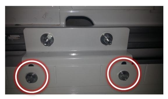
STEP 14. Loosely assemble L-bracket for the end straps to the carriage bolt/plate assembled in STEP 8. L-brackets and end straps are included with the shelf. Use washer and 5/16-18 nylon lock nut using 1/2" socket. The face of the L-bracket that is perpendicular to the mounting channel may face front or rear of the van depending on the shelf size and configuration.
