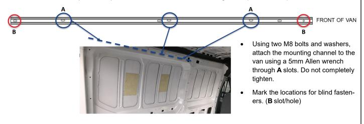
STEP 2c. Mount Rear (driver side) channel for 148" extended wheelbase high roof (975105-3-01).
