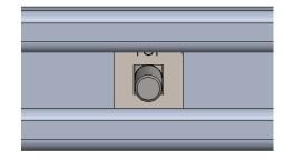
**STEP 10.** Position the shelves and carriage bolts/plates in desired location and fasten the shelves to the carriage bolt/plate using 5/16-18 nylon lock nuts and washers using 1/2" socket. Fine tune the position and alignment of the shelves in desired location. Torque them down to 13 ft-lbs.
