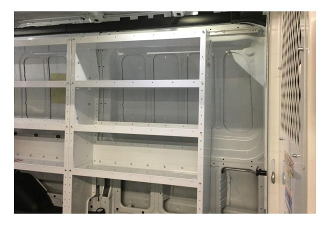
STEP 7. Assemble two mounting brackets to the back of the top shelf lip on outer-most position shown below using two 1/4-20 x 3/4" bolts, washers, and nylon lock nuts. Use 3/4" and 3/8" spacers with 1/4-20 x 2-1/2" bolts when the end panel interferes with the C-pillar on the driver side. Do not torque them down at this point.
