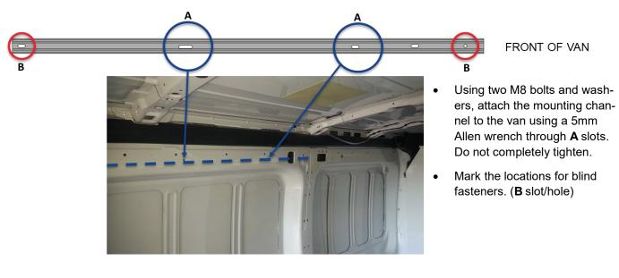
STEP 2b. Mount Rear (driver side) channel for 148" wheelbase mid/high roof (975104-3-01).
