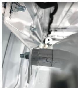
Position the carriage bolt plate such that you can read the word "TOP" and insert 5/16-18 carriage bolt from the bottom of the plate. Note: using a piece of masking tape (or equivalent) on back of the plate to lightly hold the carriage bolt to the plate may allow easier installation. You will need four plates per shelving unit plus two for each side (driver/passenger) for the end straps.
