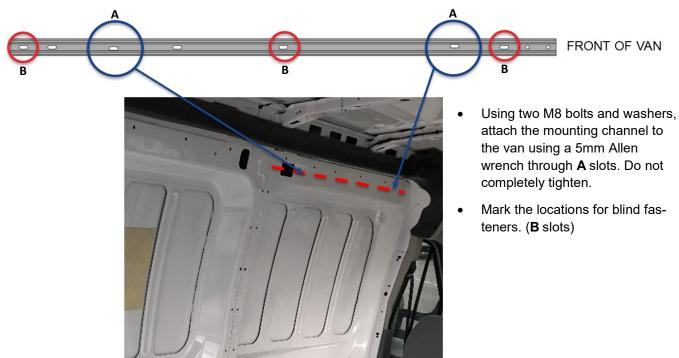
STEP 2a. Mount Rear (driver side) channel for 130" wheelbase mid/high roof (975103-3-01).
