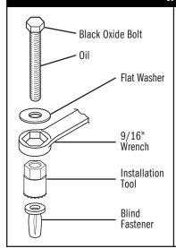
Place a drop of oil on the black oxide bolt before assembling as shown on right.
