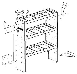
**STEP 7.** Check for shelf unit alignment and straightness and after making any adjustments, tighten the M6-1.0 bolts and lock nuts to 10 ft-lbs. using the 10mm socket, a driver and the torque wrench. Then using the 17mm socket and a driver, tighten the M10-1.5 bolts to 15 ft-lbs.
