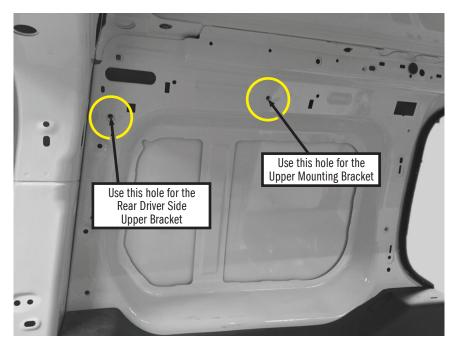
Attach one Upper Mounting Bracket to the weld nut in the center of the side panel using  $(1) M6-1.0 \times 16 mm$  bolt and (1) flat washer with a 10 mm socket and driver.
