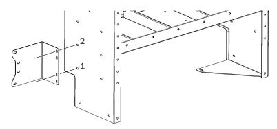
**STEP 6.** Place the 36" wide shelf unit in the van and fit it to the mounting brackets and mounting foot.
