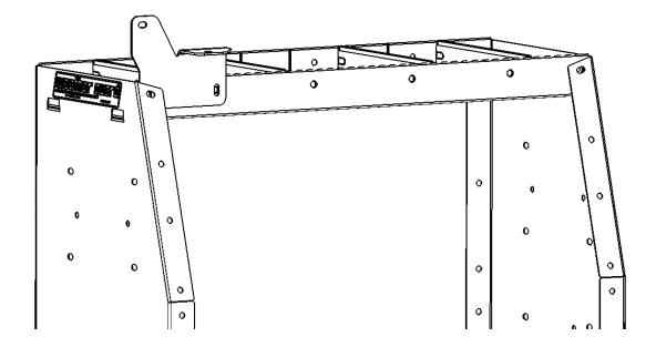
**STEP 10.** Install the Front Mounting Foot on the same end panel using (2) M6-1.0 x 16mm bolts, (2) flat washers, and (2) M6-1.0 lock nuts.
