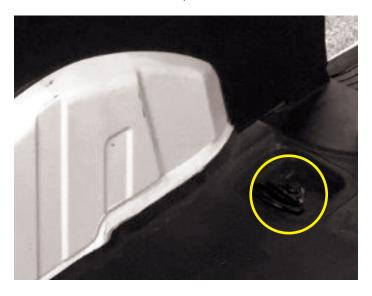
**STEP 2.** Starting on the driver side, mount the Driver Side Mid Mounting Foot to the van floor using (1) M10-1.5 x 40mm bolt and (1) 12.7mm thick floor spacer. Use the 17mm socket and driver to loosely attach the mounting foot. **Do not completely tighten at this time, allowing the foot to pivot about the mounting bolt.** Repeat with the Curb Side Front Mounting Foot.
