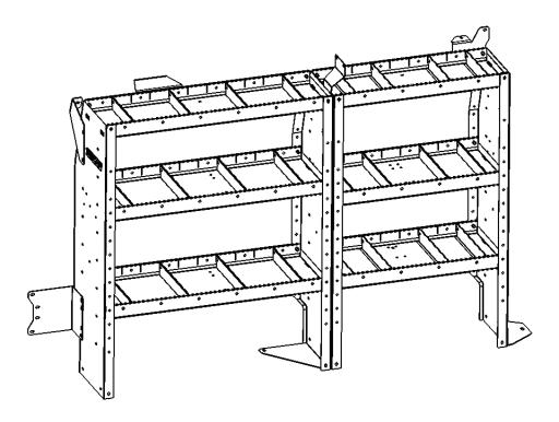
**STEP 12.** The flat part of the Front Upper Bracket will line up to an existing hole and the bent tab of the Front Upper Bracket will line up to an untapped weldnut. Through-bolt the flat part to the existing hole using M6-1.0 x 16mm bolt, nylon lock nut, and a washer and tighten. Install the M6.3-1.8 x 19mm Self-Tapping Screw through the untapped weldnut. Do not overtighten.
