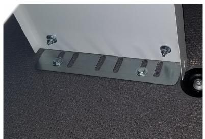
STEP 13. Torque down the 1/4-20 x 3/4" bolts, washers, and nylon lock nuts installed in STEP 7 to 76 in-lbs.
