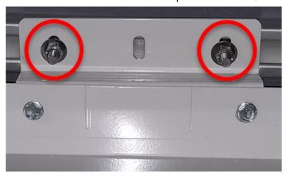
**STEP 11.** Place the mounting foot to the inside of the end panel and mark drilling points. Use a spacer when mounting on uneven surface as shown below. Use a 1" hole saw if the van is equipped with floor mats. Use a 1/4" drill bit for pilot and 3/8" drill for 1/4-20 blind fasteners. Install 1/4-20 blind fasteners on the floor. Refer to blind fastener instruction on page 5. **Always be sure to make sure you won't be damaging wiring, gas lines, or other critical vehicle systems when drilling**.
