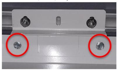
**STEP 14.** Loosely assemble L-bracket for the end straps to the carriage bolt/plate assembled in **STEP 8.** Use washer and 5/16-18 nylon lock nut using 1/2" socket. The face of the L-bracket that is perpendicular to the mounting channel may face front or rear of the van depending on the shelf size and configuration.
