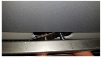
Angle the front end of each plate into its respective obround and push them toward the front of the van until their back end can be pushed into the obround.
