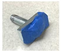
STEP 9. Insert the carriage bolt/plate assemblies through the mounting channel and rotate 90 degrees clockwise. Ten will be used on driver side and six will be used on passenger side when installing standard configuration of two and one shelving for driver side and passenger side, respectively. Note: 170" wheelbase vans use three shelves on the driver side, thus, will require 14 carriage bolts/plates on driver side.
