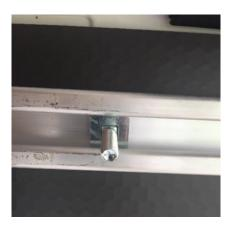
**STEP 10.** Position the shelves and carriage bolts/plates in desired location and fasten the shelves to the carriage bolt/plate using two 5/16-18 nylon lock nuts and washers using 1/2" socket. (Use outer two bracket slots if possible, but the middle bracket slot can be used if one of the outer slots causes interference) Fine tune the position and alignment of the shelves in desired location. Torque them down to 13 ft-lbs.
