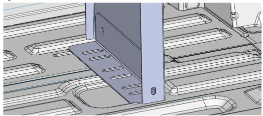
STEP 12. Slip the mounting foot from the other side of the end panel and install using 1/4-20 x 3/4" bolts, washers, and nylon lock nuts. Install to floor blind fasteners using 1/4-20 x 1-1/2" bolts. Repeat steps 11 and 12 until all mounting feet are installed. Note that you only need to use one mounting foot where the driver side shelves join.
