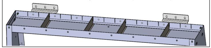
STEP 8. Position the carriage bolt plate such that you can read the word "TOP" and insert 5/16-18 carriage bolt from the bottom of the plate. Note: using a piece of masking tape (or equivalent) on back of the plate to lightly hold the carriage bolt to the plate may allow easier installation. You will need four plates per shelving unit plus two for each side (driver/passenger) for the end straps.
