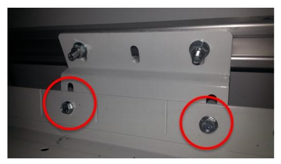
**STEP 15.** Loosely assemble L-bracket for the end straps to the carriage bolt/plate assembled in **STEP 9.** Use washer and 5/16-18 nylon lock nut using 1/2" socket. The face of the L-bracket that is perpendicular to the mounting channel may face front or rear of the van depending on the shelf size and configuration.
