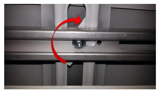
• Once all the bolts in the channel are tight, tighten the bolts holding the brackets to the upper lip of the van. Torque to 76 in-lbs.
