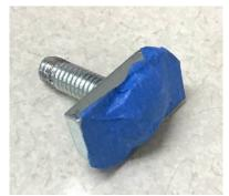
STEP 10. Insert the carriage bolt/plate assemblies through the mounting channel and rotate 90 degrees clockwise. Ten will be used on driver side and six will be used on passenger side when installing standard configuration of two and one shelving for driver side and passenger side, respectively.
