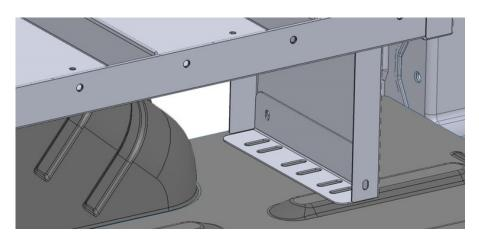
STEP 13. Slip the mounting foot from the other side of the end panel and install using 1/4-20 x 3/4" bolts, washers, and nylon lock nuts. Install to floor blind fasteners using 1/4-20 x 1-1/2" bolts. Repeat steps 12 and 13 until all mounting feet are installed. Note that you only need to use one mounting foot where the driver side shelves join.
