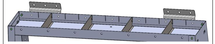
STEP 9. Position the carriage bolt plate such that you can read the word "TOP" and insert 5/16-18 carriage bolt from the bottom of the plate. Note: using a piece of masking tape (or equivalent) on back of the plate to lightly hold the carriage bolt to the plate may allow easier installation. You will need four plates per shelving unit plus two for each side (driver/passenger) for the end straps.
