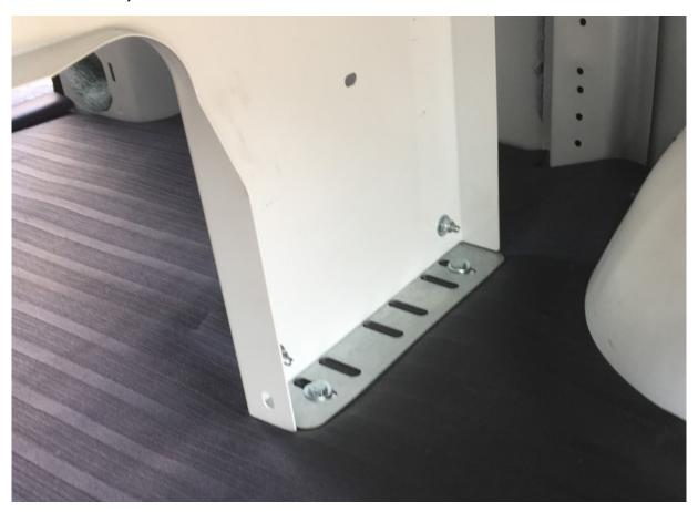
**STEP 14.** Torque down the 1/4-20 x 3/4" bolts, washers, and nylon lock nuts installed in **STEP 8** to 76 in-lbs.
