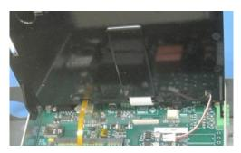
3. Connect the 4-pin ribbon cable to the TOUCH SCREEN connector.
