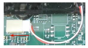
6. Insert the 2-pin stacker display ground in the J-18 connector.
