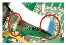
Make sure the tabs on each side are up when you connect the ribbon cable. Lock each side of the connector, alternating back and forth until both are seated properly. Gently tug the ribbon cable after you lock the tabs to verify that the white ribbon cable is locked in place.
