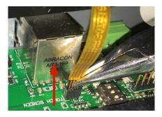
**IMPORTANT:** In the following step, be extremely careful and gentle when you remove the large, white ribbon cable. The connector is very delicate. If you break it, you must replace the entire main circuit board.
