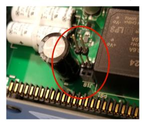
4. Remove the 4-pin ribbon cable from the TOUCH SCREEN connector on the main circuit board.
