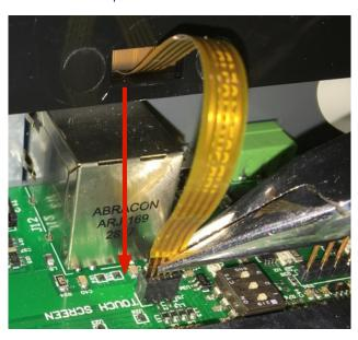
**IMPORTANT:** In the following step, be extremely careful and gentle when you connect the large, white ribbon cable. The connector is very delicate. If you break it, you must replace the entire main circuit board.
