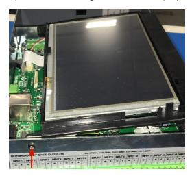
8. Pivot the display assembly until the other hinge tab is disengaged, and then lift out the display assembly.
