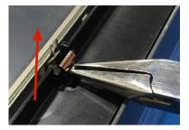
2. Press in one of the side tabs on the display until it is disengaged, and then press in the other side tab. Flip the LCD display up when both side tabs are disengaged.
