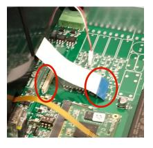
6. Remove the 2-pin backlight cable from the BACKLIGHT connector.
