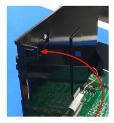
3. Gently grasp the 2-pin stacker display ground with your fingers or smooth jaw, needle nose pliers, and then gently pull straight up out of the J18 connector. If the stacker is bent, discard it. If it is not bent, save it as a spare part.
