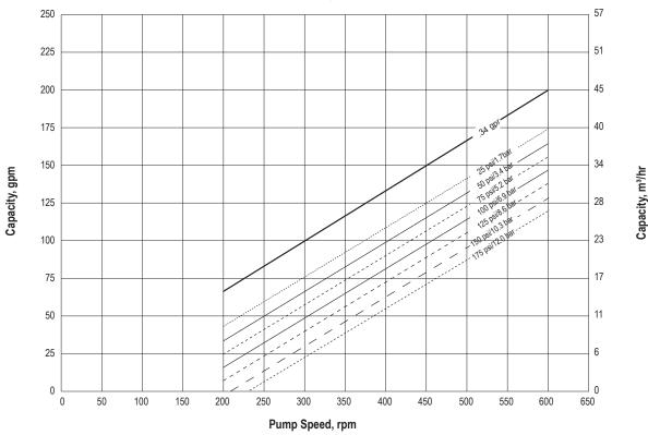
\*Note: Output from lobes coated with elastomers other than NBR maybe lower. Contact Engineering for further information.
