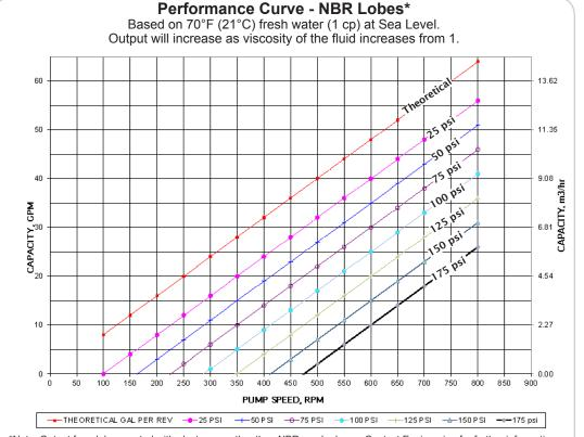
\*Note: Output from lobes coated with elastomers other than NBR maybe lower. Contact Engineering for further information.
