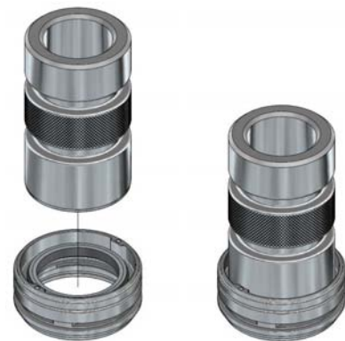
Fig. 10.4.4 Installation of the mechanical face seal using the Face Seal Pusher tool.
