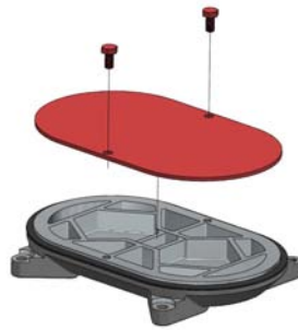
Fig. 10.3.1.1 “No hole” cover wear plate installation
