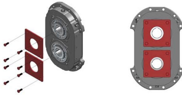
Fig. 10.3.2.8 Installation of the bearing / sleeve locking plates
