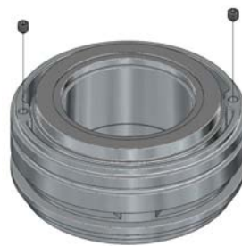
Fig. 10.1.5.7 Reinstallation of the seal holder set screws
