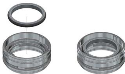
Fig. 10.4.3 Insertion of the face seal and O-ring
