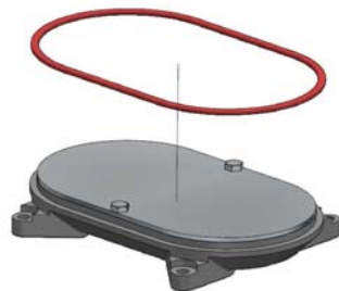
Fig. 10.3.1.3 Pump cover O-ring installation
