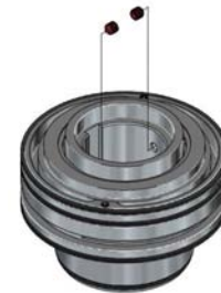
Fig. 10.3.2.2 Installation of the shaft sleeve set screws
