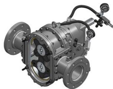
Fig. 10.5 Reference seal pressure test assembly
