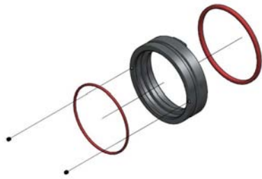
Fig. 10.3.2.3 Installation of the lobe spacer O-rings
