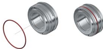
Fig. 10.2.1.2 Installation of external secondary O-rings
