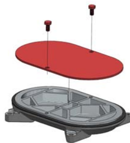
Fig. 10.1.2 Removal of the pump cover wear plate (standard frame only)
