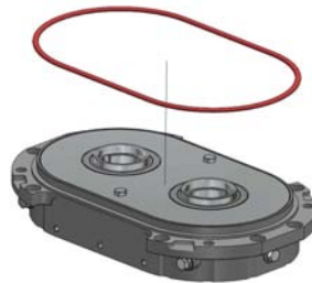
Fig. 10.3.2.9 Installation of the high pressure door O-ring
