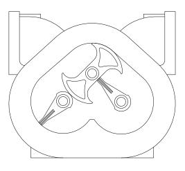
The rotors in the meter are designed to operate at close tolerances to one another and the wall of the fluid chamber. There are slight clearances between the rotors and the chamber wall. Because of this, it is important that the meter be properly applied for the flow rate and operating pressure of the system.
